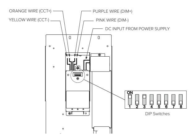
The LED panels can be connected to the controller outputs as shown below:
